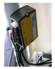
To fix the interface to the cage use provided cable ties. Remember that you should easily reach the white main power connector, to switch off safety/tracking devices at the end of racing day. Important: do not squeeze wires with to much fastened cable ties, when fixing them to rollbar and leave last
